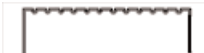
Vinyl Tile and Vinyl Plank (over non-porous substrates) 1/16" x 1/32" x 1/32" U notched Approx. 300 sq. feet/gallon spread rate
