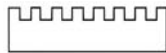
Vinyl Tile and Vinyl Plank (over porous substrates) DriTac trowel TR-8 1/16" x 1/16" x 1/16" square notched Approx. 160 sq. feet/gallon spread rate
