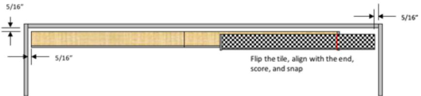
**IMPORTANT:** Inspect the cut plank to ensure the break was smooth and even. It may require shaving the backing to keep it smooth and even. Make sure there is no debris at the joints. Note: this method of cutting may lead to more cracks and breaks in the backing close to the score line, which will require use of a new plank.
