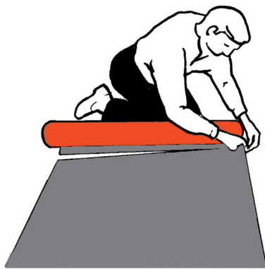
1. Roll out GamFloor™ and trim to fit with backing side up
