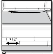
**[6]** Use a cut piece of board from the previous row to start the next row. This starting plank section must be at least 12" long. If the piece is too short, start with a new board. Cut the new board in one-third, one-half or two-thirds length sections, depending upon what is required to maintain the random stagger from one row to the next. Always ensure that the end joints are staggered at least 12 to 16 inches from one row to the next.
