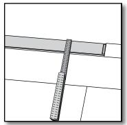
**[10]** Measure and cut the planks in the last row to fit. Remember to allow for a minimum of 1/4" expansion space from the wall.
