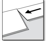
[2] In the first row, place the second plank tight against the short end of the first plank.
