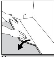
**[7]** Place the plank at an angle against the plank in the previous row. Press the edge forward against the previous row, and then fold down at the same time.
