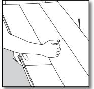
[1] Separate the whole row by carefully lifting up and releasing the whole row. Fold up and release the whole long side of the row, being very careful not to allow the planks to bend downward at the end seams! This could damage the locking mechanism of the plank!
