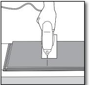
**[5]** Place the plank face down on the work surface and cut to size with a power saw. If you are using a hand saw, use a fine-toothed blade, and cut the planks face up
