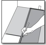
**[4]** Place the final plank face down with the short side (without the locking strip) towards the wall. The remaining expansion space should be at least a minimum of 1/4" from the wall. Draw a pencil line where the plank is to be cut.
